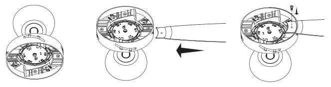
**WARNING**: This Fan has click in blades, it is essential that the installing <u>electrician has applied an appropriate</u> <u>amount of force to ensure the blades are clicked in securely before engaging the screw and before turning the fan on.</u> This is to ensure the blade is secured, and in the case of a defective spring latch. Four Seasons will not be responsible for any consequential damage because of this.
