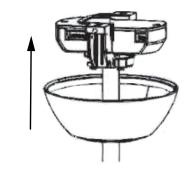
Slide the canopy upward onto the mounting bracket and rotate it counter-clockwise to lock it in place. Verify that both mounting bracket tabs are fully engaged within the canopy slots. The canopy should have an approximate 3mm gap from the ceiling.
