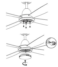
Align the convex point on the light plate with the gap on the LED mounting plate and press down firmly.
