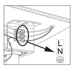
Fix the Earth cable and complete all electrical connections at the mounting bracket.
