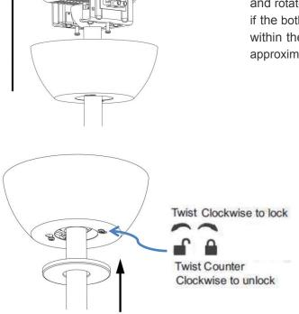
Slide the canopy upward onto the mounting bracket and rotate it counter-clockwise to lock it in place. Check if the both mounting bracket tabs are fully engaged within the canopy slots. The canopy should have an approximate 3mm gap from the ceiling.
