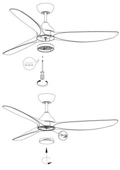
Align the convex point on the light plate with the gap on the LED mounting plate and press down firmly while twisting on.
